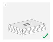
Altro Whiterock panels need to be stored flat on a pallet and not on the floor or concrete subfloor.
