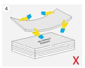
8'2" or 9'10" A large bend/bow in the panel can damage the film.
