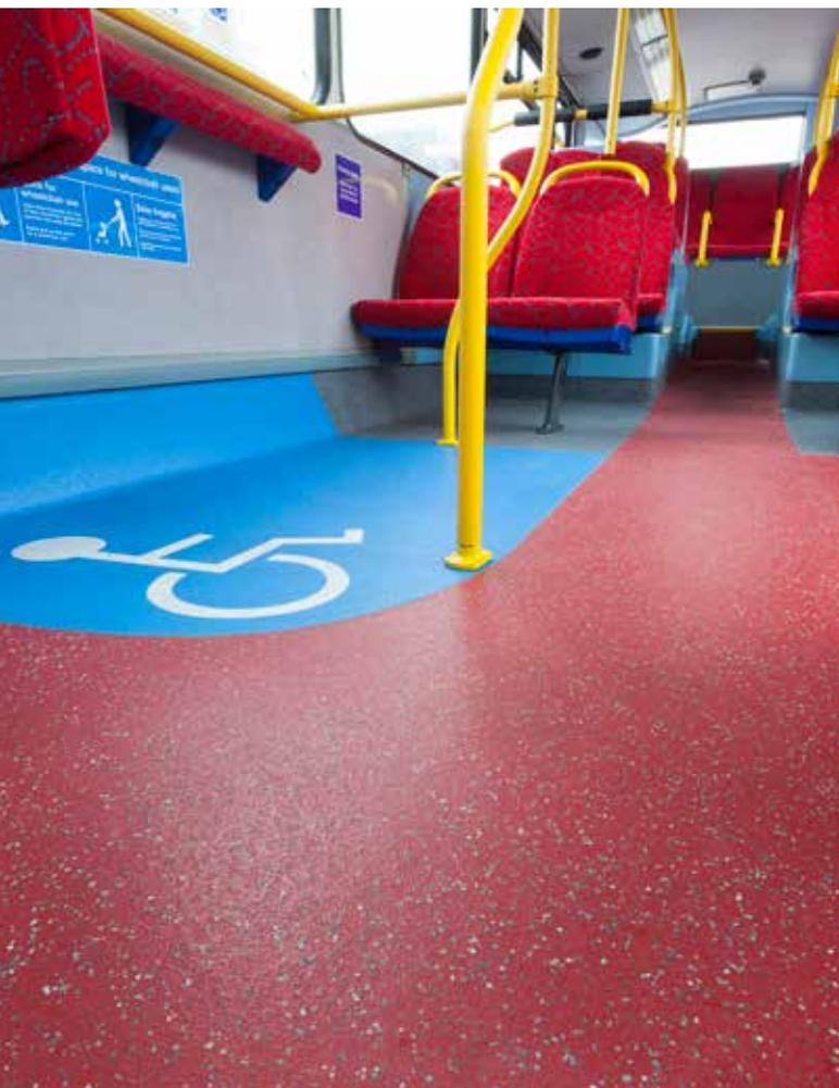
“Refurbishing the fleet of Abellio buses is quite complex. Removing the old flooring can be tricky and involves using a heat gun to melt the glue and loosen the flooring. Once that’s up, it takes around one week to install the new flooring on each bus.
