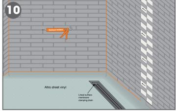
Apply Altro sanitary sealant as shown in drawing at inside corners, as well as top and bottom of all panels to prevent moisture ingress.
