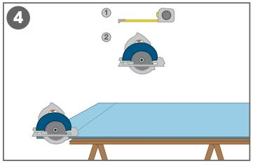
Measure and mark out the previously determined measurements onto panel. Make necessary cuts. Always dry fit to ensure proper fit.
