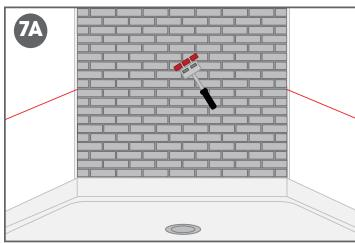
7A. If the distance was 48" or less the panel will be installed vertically. Install panel into the correct position. Use a 3 wheeled wall roller to roll entire panel to ensure proper bond to the substrate.
