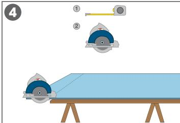
Measure and mark out the previously determined measurements onto panel. Make necessary cuts. Always dry fit to ensure proper fit.
