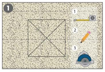
Use datum line or similar to determine location on wall substrate for placement of the Altro Whiterock Recessed Shelf A900. Measure, mark, and cut wall substrate accordingly.
