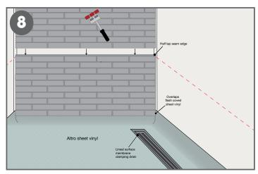
8. Install the top panel as previously instructed with correct space and properly aligned with the previously installed bottom panel. Use a 3-wheeled wall roller to roll entire panel to ensure proper bond to wall substrate.
