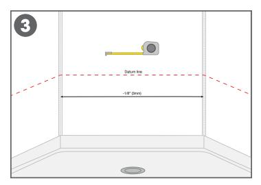
Measure distance between the A839 allowing for 1/8"(3mm) tolerance. If distance is 48" or less, the panel can be installed vertically. Any distance over 48" and in a wet area application will require the half-lap seam method. Orientation of the panels will need to be determined prior to the ordering process.
