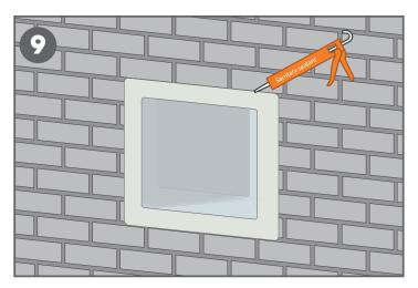
Once installation is complete, the edges of the Altro Whiterock Recessed Shelf A900 must be sealed with Altro Sanitary Sealant to prevent water ingress.
