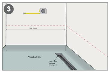
3. Measure distance between the A839 allowing for 1/8"(3mm) tolerance.
