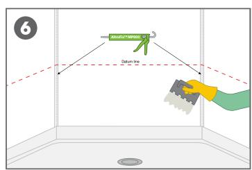
6. Depending on the environmental conditions and substrate, mixing of two-part adhesives may be necessary. Follow adhesive label and mix thoroughly. Apply adhesive to back of panel and/or to the wall substrate. Apply a bead of AltroFix™ MP600 to the internal corner of the previously installed A839 trims.
