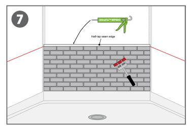
7. Install panel into proper position with correct spacing and aligned on or with datum line. Use a 3-wheeled wall roller to roll entire panel to ensure proper bond to wall substrate. Apply 1/16"(2mm) bead of AltroFix™MP600 to the half-lap seam edge. Be sure to keep it above the visible seam edge.
