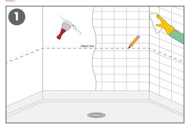
All surfaces must be smooth, sound, dry, and free of contamination Check walls for flatness especially at seam location(s). Existing wall tile must be cleaned with TSP (trisodium phosphate) or equivalent to remove soap scum and contaminates, rinsed with clean water and allowed to dry. Any loose tiles must be fixed and made sound. Lastly add a datum line with pencil.
