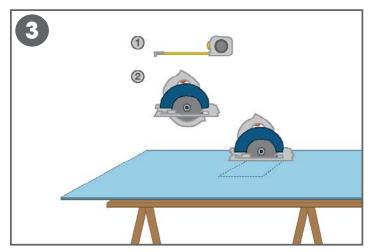
Transfer the measurements to the Altro Tegulis panel and cut the opening, which will be approximately 10 1/8" x 10 1/8" for the recessed body to fit into the cut out with ease.
