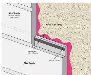
For wet areas only: Measure the inside corner(s) from top to bottom, cut the strips of A839 for each inside corner trims and adhere them using AltroFix™ MP600. Prior to installing the Altro Tegulis panels, apply a bead of AltroFix™ MP600 to the internal corner of the previously installed A839 trims.
