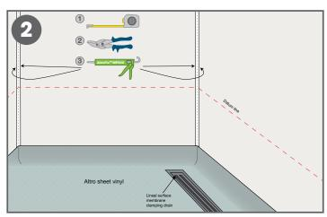
Measure the inside corner(s), cut the strips of A839 to length, and adhere them using AltroFix™ MP600.
