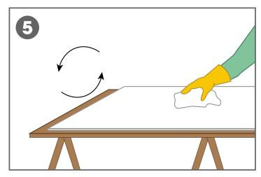
Clean the back of the panels with glass cleaner or similar to remove dust and contaminates.
