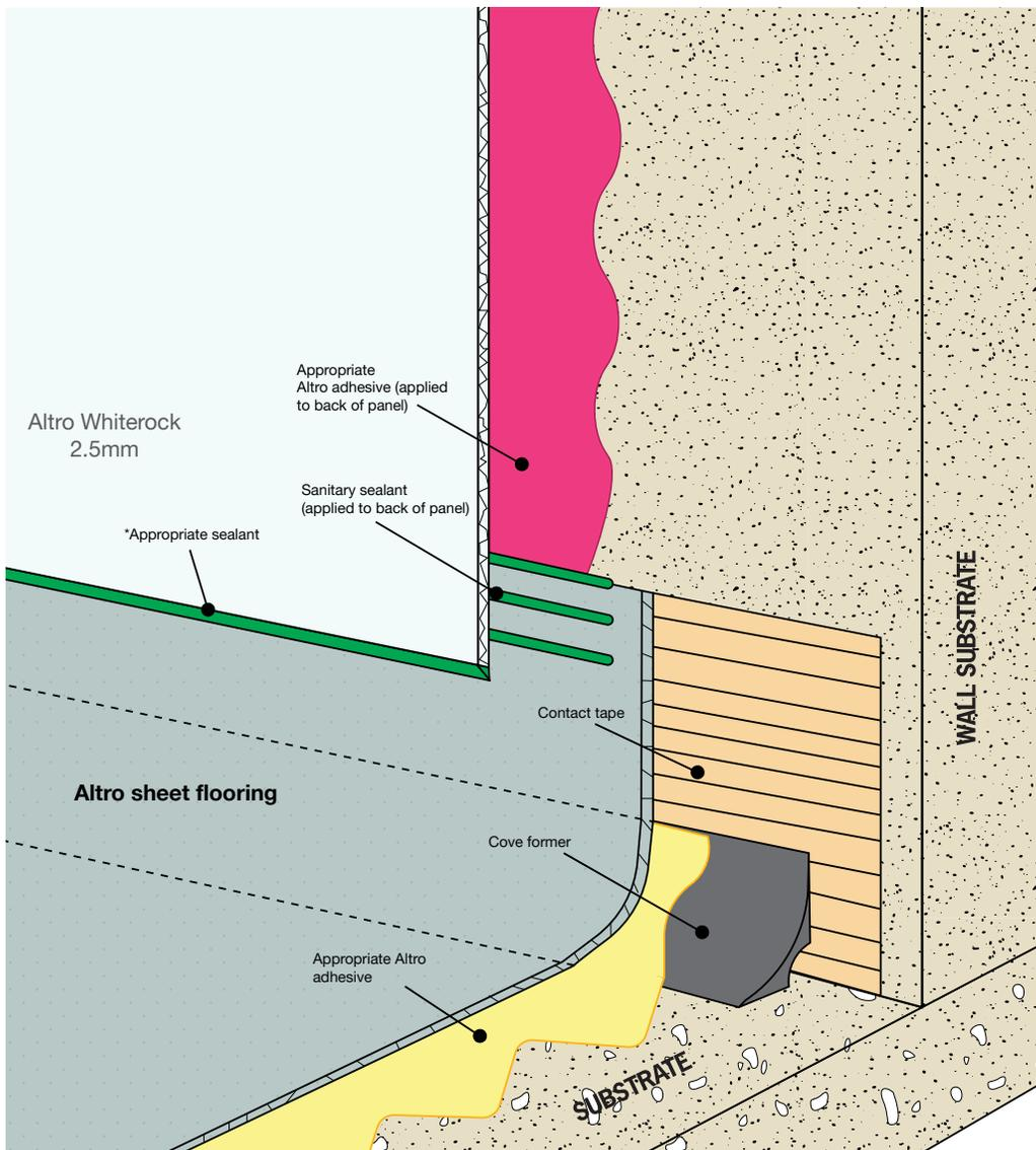
An overlap transition from floor to wall is our preferred installation method and is utilized in most installations. It is completed by installing the flooring 6" – 8" up the wall, dependent on cove size and installing the Altro Whiterock with a 2" overlap. The juncture is then finished with Altro sanitary sealant or tamper-resistant security sealant.
