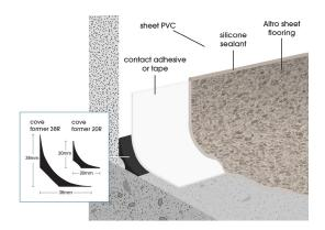
Utilising heat can aid in shaping the vinyl during coving; however, it is crucial to exercise caution to prevent burning or causing damage to the vinyl surface.
