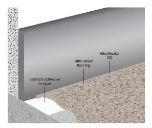
After the vinyl has been laid out and conditioned, overlap all joints by approximately 20mm and cut with the aid of a scribing tool to form a tight joint.
