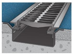
Where falls to waste are present, it is crucial to ensure the subfloor composition is suitable. Only formed concrete, engineered screeds, bulk fill reinforced levelers, or products designed and warranted for such applications should be used. Installation over sand-cement screeds should not
