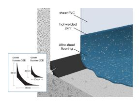
The use of heat will assist in forming the vinyl when coving, but all care must be taken to avoid burning or damaging the vinyl surface. Caution should always be exercised when using flammable solvent-based adhesive and a gas torch simultaneously. It is essential to adhere to all manufacturers safety requirements and guidelines to minimize any potential risks or hazards.
