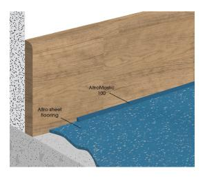
After the vinyl has been laid out and conditioned, overlap all joints by approximately 20mm and cut with the aid of a scribing tool to create a consistent 0.5mm gapped joint. Whether the joints are cut in before or after applying the adhesive can be based on the preference of the flooring installer. However, in large installations, it is important to consider that cutting the joints and perimeter beforehand may create
