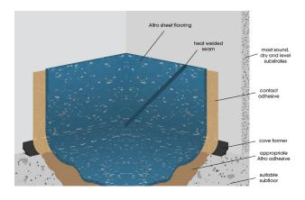
Allow 12 hours between laying and welding to ensure adhesive is properly set.
