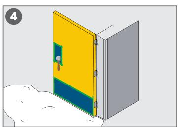
4. Once the adhesive is dry, position the push plate and/or kick plate. Roll entire plate(s) with a hand roller to ensure it is fully adhered.
