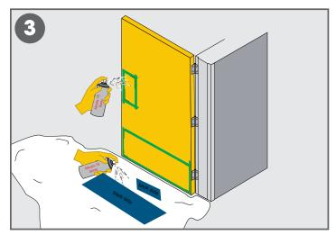
3. Use a drop cloth and mask the surrounding door surface to protect from overspray. Spray the backside of each push plate and/or kick plate as well as the door surface with AltroFix 75 Spray. Hold can 6"-10" from material. Allow adhesive to dry to the touch.
