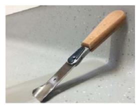
11. Trim welded seam with toe trimming knife (AST TTRIMMER).
