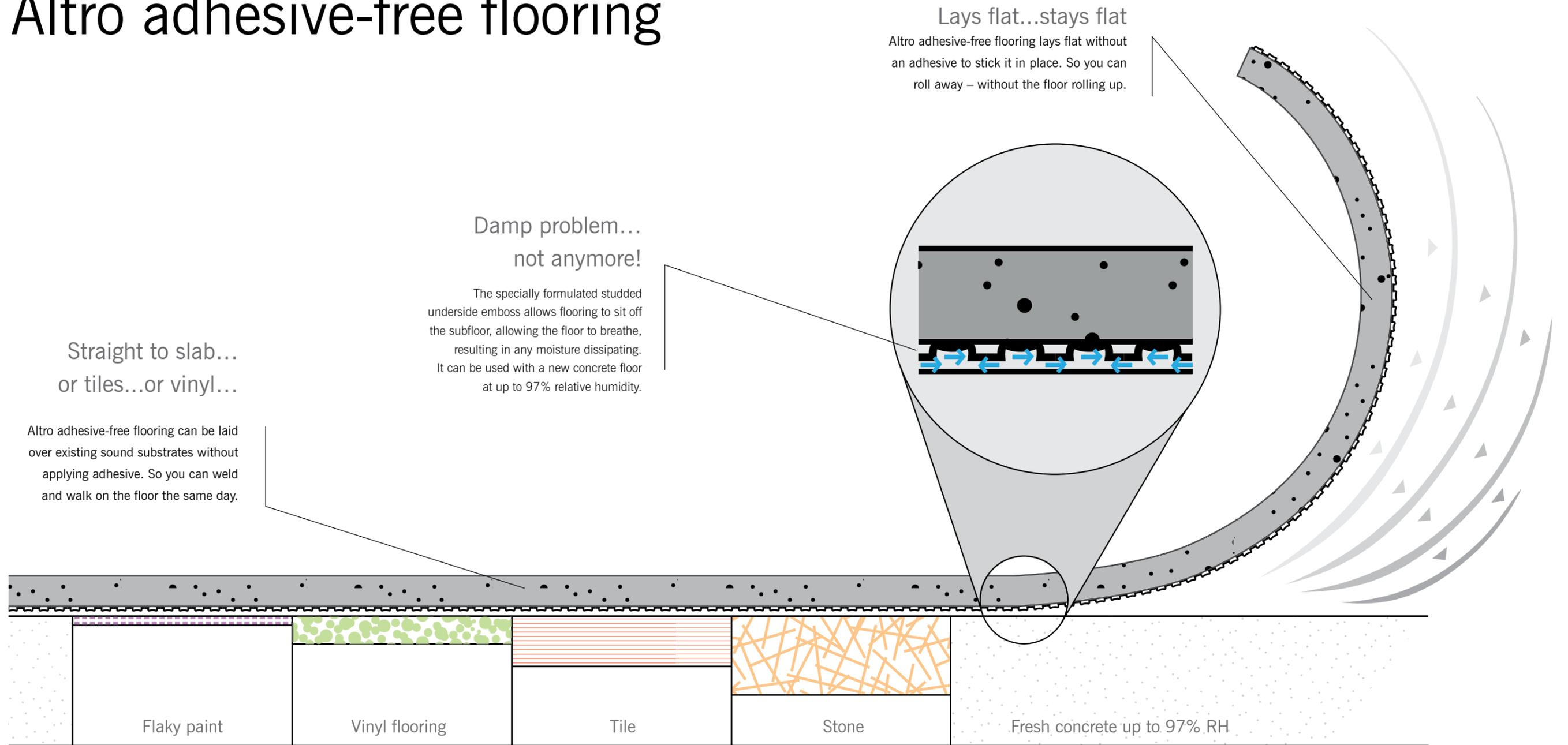
Altro adhesive-free flooring gives a quick fit without compromising on safety or durability. Its unique formulation allows the floor to lie flat and perform like a traditional adhered safety floor **without the need for an adhesive**.
