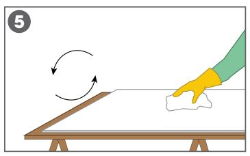
5. Clean the back of the panels with isopropyl or denatured alcohol to remove dust and contaminates.
