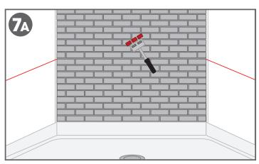
7A. If the distance was 48" or less the panel will be installed vertically. Install panel into the correct position. Use a 3 wheeled wall roller to roll entire panel to ensure proper bond to the substrate.
