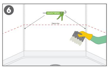
6. Depending on the environmental conditions and substrate, mixing of two part adhesives may be necessary. Follow adhesive label and mix thoroughly. Apply adhesive to back of panel and/or to the wall substrate. Apply a bead of AltroFix™MP600 to the internal corner of
