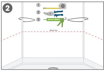
Measure the inside corner(s), cut the strips of A839 to length, and adhere them using AltroFix™MP600 adhesive.
