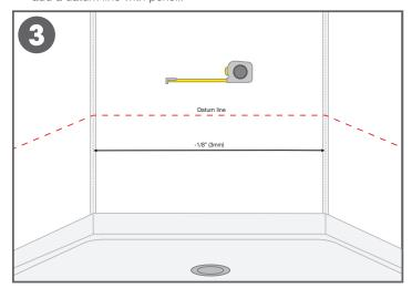
3. Measure distance between the A839 allowing for 1/8"(3mm) tolerance. If distance is 48" or less, the panel can be installed vertically. Any distance over 48" and in a wet area application will require the half-lap seam method. Orientation of the panels will need to be determined prior to the ordering process..
