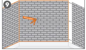
9. Side wall panels can be installed vertically which will need to be determined prior to the ordering process. This allows full panels to be installed without any seams. This is recommended only if the wall is less than 48"wide. Install adjacent panels as previously instructed. Apply Altro sanitary sealant as shown in drawing at inside corners, as well as top and bottom of all panels to prevent moisture ingress.
