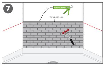
7. Install panel into proper position with correct spacing and aligned on or with datum line. Use a 3 wheeled roller to roll entire panel to ensure proper bond to wall substrate. Apply 1/16"(2mm) bead of Parabond 600 adhesive to the half lap seam edge. Be sure to keep it above the visible seam edge.
