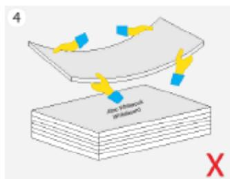
A large bend/bow in the panel can damage the film.
