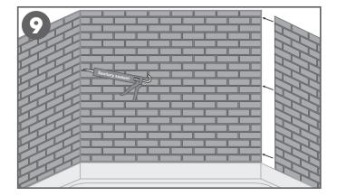
Side wall panels can be installed vertically which will need to be determined prior to the ordering process. This allows full panels to be installed without any seams. This is recommended only if the wall is less than the panel width. Install adjacent panels as previously instructed. Peel back the protective film at the inside corners as well as top and bottom of all panels and apply a bead of colour coordinated Altro sanitary sealant as shown in drawing to prevent moisture ingress.
