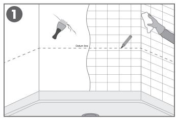
All surfaces must be smooth, sound, dry, and free of contamination. Check walls for flatness especially at seam location(s). Existing wall tiles must be cleaned to remove soap residue and contaminants, rinsed with clean water and allowed to dry. Any loose tiles must be fixed and made sound. Lastly add a datum line with pencil.
