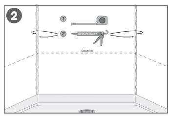
Apply a bead of Altro sanitary sealant to the substrate vertically on both sides of the corner where the sheets are to be installed.
