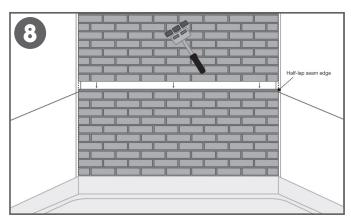
8. Install the top panel as previously instructed with correct space and properly aligned with the previously installed bottom panel. Use a 3 wheeled roller to roll entire panel to ensure proper bond to wall substrate.
