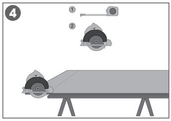
Measure and mark out the previously determined measurements onto the panel. Make any necessary cuts. Dry fit to ensure proper fit
