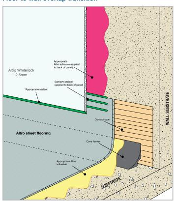
An overlap transition from floor to wall is our preferred installation method and is utilized in most installations. It is completed by installing the flooring 6"-8" up the wall, dependent on cove size and installing the Altro Whiterock with a 2" overlap. The juncture is then finished with Altro sanitary sealant or tamper-resistant security sealant.
