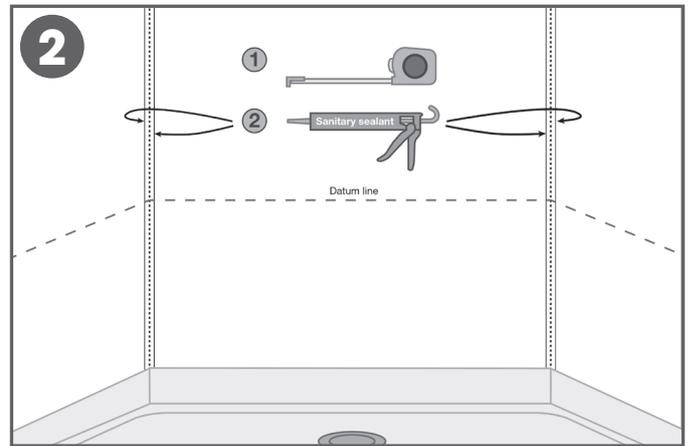
2. Apply a bead of Altro sanitary sealant to the substrate vertically on both sides of the corner where the sheets are to be installed.
