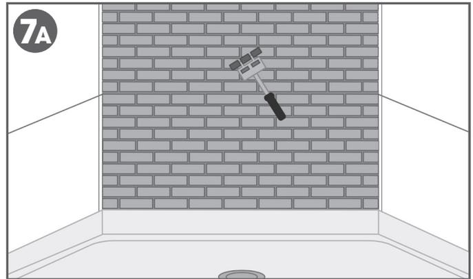
7A. If the distance is less than the panel width, it can be installed vertically (dependent on design). Install panel into the correct position. Use a 3 wheeled wall roller to roll entire panel to ensure proper bond to the substrate.
