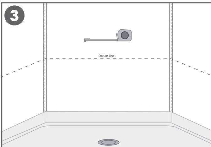
3. Measure distance between corners allowing for a 2mm tolerance in each corner. Any distance over the width of a single sheet and in a wet area application will require the half-lap seam method. Orientation of the panels will need to be determined prior to the ordering process.
