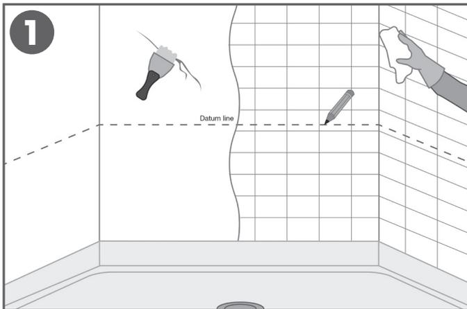
1. All surfaces must be smooth, sound, dry, and free of contamination. Check walls for flatness especially at seam location(s). Existing wall tiles must be cleaned to remove soap residue and contaminants, rinsed with clean water and allowed to dry. Any loose tiles must be fixed and made sound. Lastly add a datum line with pencil.
