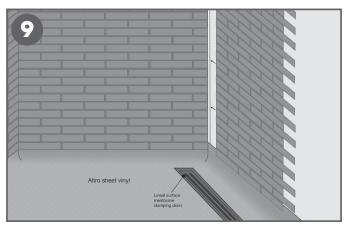
9. Additional wall panels that are not in direct contact with continuous moisture can be installed vertically with the interlocking joining method. This allows full panels to be installed without any horizontal seams. Install adjacent panels as previously instructed.
