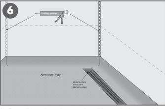
Depending on the environmental conditions and substrate, mixing of two-part adhesives may be necessary. Follow adhesive label and mix thoroughly. Apply AltroFix adhesive to back of panel.
