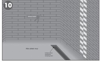
10. Peel back the protective film at the inside corners as well as top and bottom of all panels and apply a bead of colour coordinated Altro sanitary sealant as shown in drawing to prevent moisture ingress. Note: Once installation is complete, remove protective film and clean with Altro anti-static solution. Leave for 24 hours prior to being put into use.
