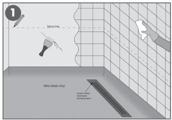
All surfaces must be smooth, sound, dry, and free of contamination. Check walls for flatness especially at seam location(s). Existing wall tiles must be cleaned to remove soap residue and contaminants, rinsed with clean water and allowed to dry. Any loose tiles must be fixed and made sound. Lastly add a datum line with pencil.
