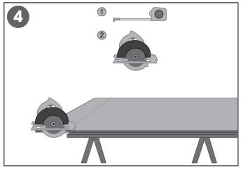
Measure and mark out the previously determined measurements onto the panel. Make necessary cuts. Always dry fit to ensure proper fit.
