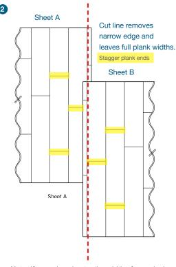
Note: If reversing sheets, the width of one plank width may need to be cut off and removed in order to keep a random pattern. This is to be determine by those on site.
