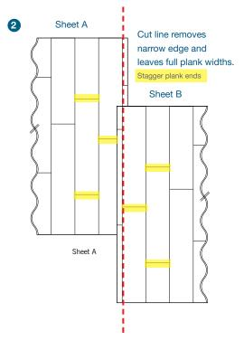
Note: If reversing sheets, the width of one plank width may need to be cut off and removed in order to keep a random pattern. This is to be determine by those on site.
