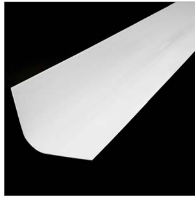
R-shape internal radius corners A940 / 25 Installed horizontally at wall and ceiling locations (ceiling to wall cove corner) and vertically on the wall at inside corners (wall cove corner). 6" x 6" x 8'2" with 2" radius.
