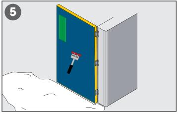
5. Once the adhesive is dry, position the door fascia in place. Roll entire panel with a hand roller to ensure it is fully adhered.
