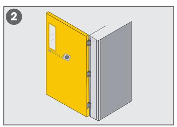
Take measurements of door as well as window locations, if applicable, as the panel must leave a 1/16" reveal. AFT Fascia will come precut with window reveal. Dry fit panel to ensure proper fit, make adjustments if necessary.
