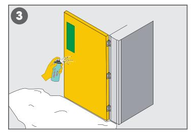
Use a drop cloth and also mask the window and surrounding door area to protect from overspray. Spray the door surface with AltroFix 75 Spray. Hold can 6"-10" from material. Allow adhesive to dry to the touch.
