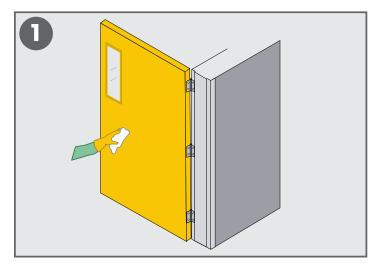
Start off by cleaning the door surface. The substrate must be clean and dry, free from dust, dirt, grease, oils, solvents, loose paint or any other contaminants.
