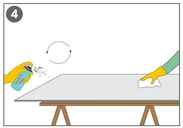
Clean the back of the panel with isopropyl alcohol or similar to remove dust and contaminates. Next use AltroFix 75 spray adhesive on entire back side of panel. Allow adhesive to dry to touch.
