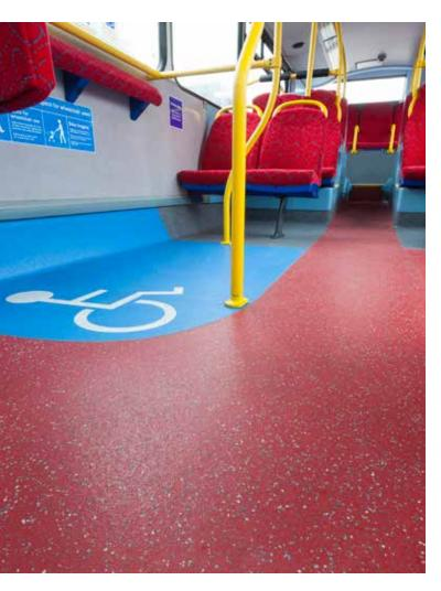
"Refurbishing the fleet of Abellio buses is quite complex. Removing the old flooring can be tricky and involves using a heat gun to melt the glue and loosen the flooring. Once that's up, it takes around one week to install the new flooring on each bus.
