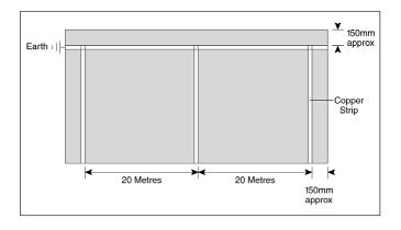
The first copper / brass strip (0.1mm thick), should be laid 150mm in from the perimeter of the room, running in the same direction as the sheet flooring. This strip should be connected to a known earth by a qualified electrician; two connections to earth are advised, the second as a backup in case the first is damaged or disconnected.
