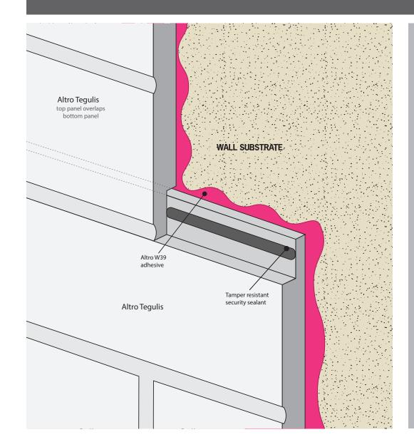
Apply an approximately 1/8° bead of tamper-resistant security sealant as shown in the detail diagram. Be sure to immediately clean up any excess sealing.
